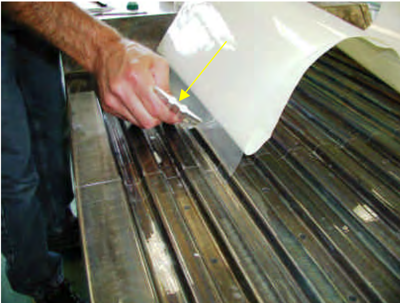
Figure 3 Film Application: use small hard plastic squeegee in tight corners and pressing out wrinkles
