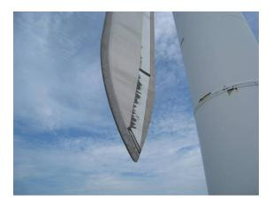
Damage to Tape and Peeling At End of Blade
